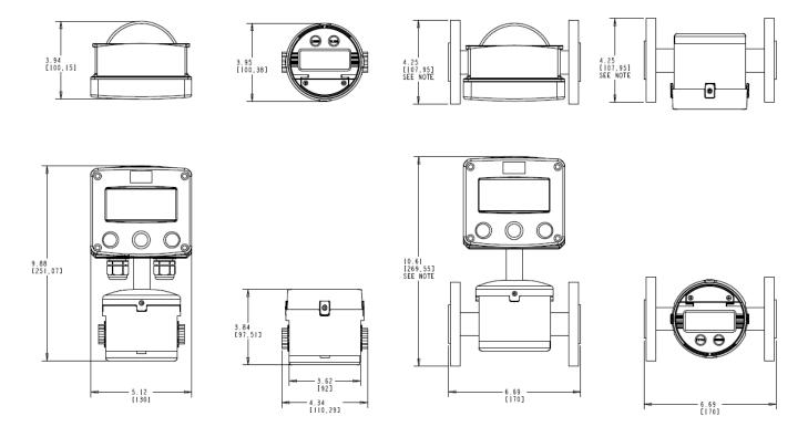
FLANGED DIMENSIONS ARE BASED OFF A 1' STAINLESS STEEL CLASS 150 FLANGE - OD OF FLANGE WILL VARY WITH METER SIZE AND FLANGE CLASS/MATERIAL - LAY LENGTH REMAINS 170mm FOR ALL FLANGED VARIATION:
